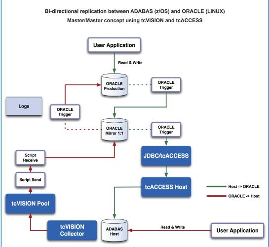
This is a simplified representation of the replication scenario between the z/OS mainframe with ADABAS and the LINUX platform with ORACLE.
